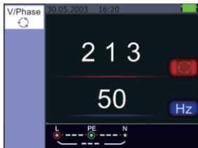
Phase Sequence Screen When connected in counter-clockwise manner
