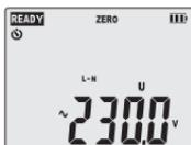
4. Press the **START/ENTER** Button to begin the measurement. Read the measurement results and press the **◀MODE or ZERO▶** Button to view other results.
