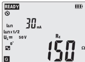
Protective Conductor Resistance for RCD- $R_E$
