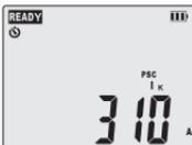
When the LCD displays “READY,” press the **START/ENTER** Button to perform the measurement again. Press the **ESC** Button to exit and return to the measured voltage.
