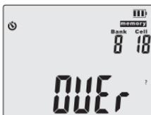
4. Press the **Memory** Button to overwrite the result or the **ESC** Button to cancel the operation.
