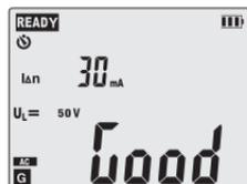
8. Use the **ENTER** Button to save the results in memory, the **MODE** and **ZERO** to view the result components or the **ESC** Button to go to the voltage display mode.
