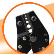
Hexagon terminal sizes: 1.5mm 2 ; 2.5mm 2 ; 4.0mm 2 ; 6.0mm 2
