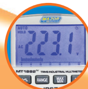
6000 Count Backlit LCD Display with 61 segmented bargraph
