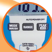
Inrush Current, Peak Hold & VFD Measurements
