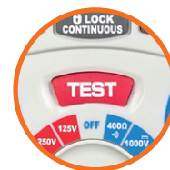
Lock down test button for continuous use
