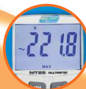
40 000 Count Backlight Display with 41 segmented bargraph
