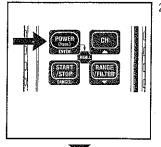
2. Press the button at least 1 sec. to power on the instrument. Release the button when all indications are displayed on the LCD.
