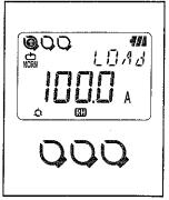
3. Check the connected Sensors. Sensor (P.7) and the full-scale value are displayed.
