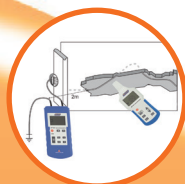
Tracking of underground and buried circuits
