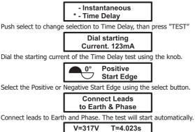
Test in progress since 4.023s. The voltage between leads is 317V and constant current is 125mA  $\,$
