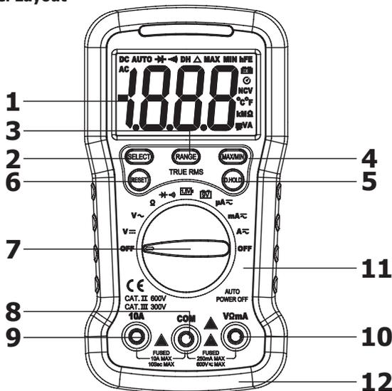
1. LCD display: 3 1/2 digits LCD display, full function symbol display.
