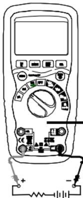
4. For current measurements up to 10A DC, set the function switch to the **10A** position and insert the red test lead banana plug into the **10A** jack, press mode button to select AC or DC.
